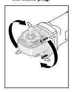
The machine head can be rotated with respect to the machine housing in 90° steps. In this manner, the On/Off switch can be brought into a more convenient position for special working situations, e.g. for left-handed persons.
