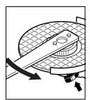
A properly attached, undamaged quick-clamping nut can be loosened by hand when turning the knurled ring in anticlockwise direction.
